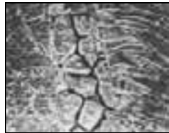
Figure 2.5: Intergranular Corrosion ( www.corrosion-club.com )
